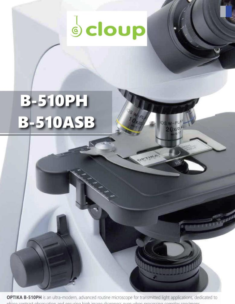
**OPTIKA B-510PH** is an ultra-modern, advanced routine microscope for transmitted light applications, dedicated to phase contrast observation and ensuring high image sharpness even when processing complex specimens. **B-510ASB** works accordingly to the international regulations about Asbestos testing, with focusable 12.5x eyepieces, and a Walton & Becket graticule to perform perfect fibers analysis at a glance.
