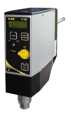
The universal laboratory stirring motor for rheometric tests. Powerful microprocessor controlled (fuzzy logic) stirrer for optimum performance and accuracy with a maximum torque of 250 Ncm, hollow shaft and precision chuck of 10.5 mm. A multi-step safety system carries out a self test of all safety functions and detects and protects against overload as well as overtemperature.
